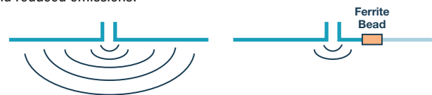
Figure 6. Use of ferrite bead to reduce effective dipole.
